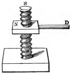
The power of the screw depends on the distance between the threads. The closer the threads of the screw, the greater will be the power; but then the number of revolutions made by the handle, D, will also be proportionably increased: so that we return to the general principle—what is gained in power is lost in time. The power of the screw may also be increased by lengthening the lever, D, attached to the nut.
