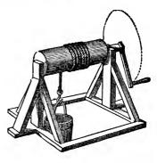
Rule.—The power to the weight, as the radius of the uxle, to the length of the crank, or radius of the wheel.
