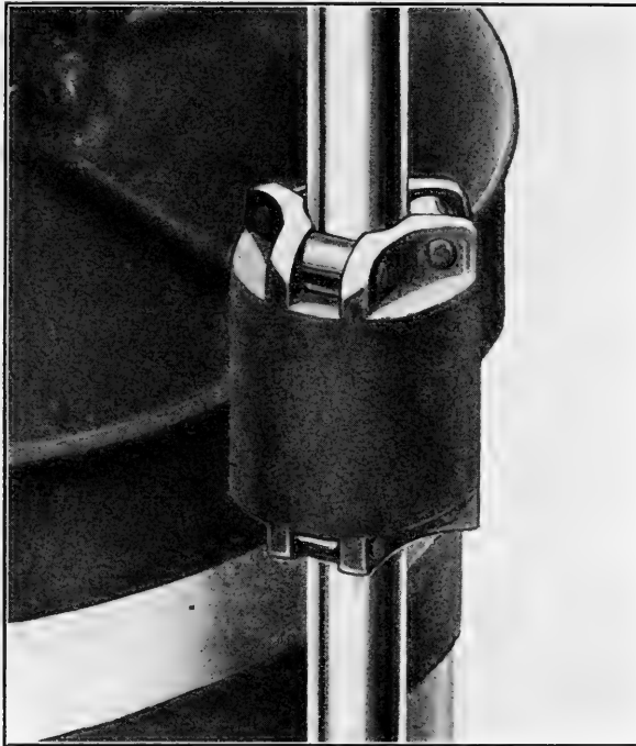
Fig. C. Sleeve of headpiece on standard, with steel rollers above and below. \times \frac{1}{2} .
