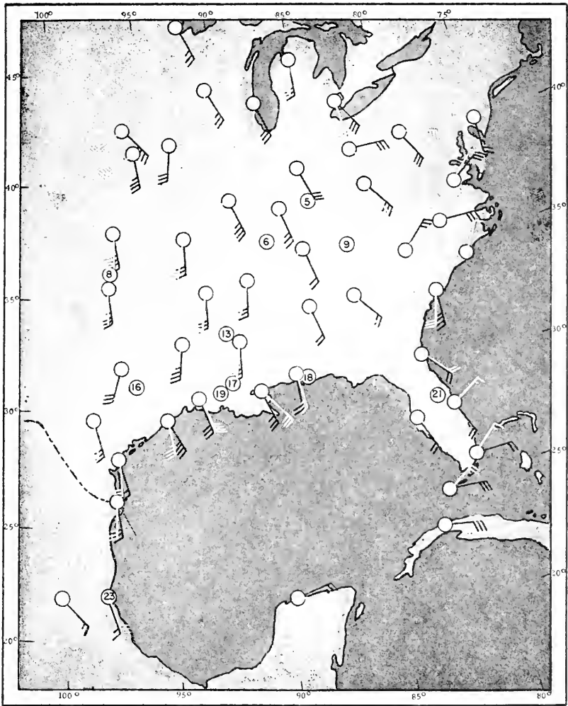
FIG. 45. Winds aloft at 10:00 P. M. on April 24 (CST). Winds at 2,000 feet above mean sea level are shown in black; those at 4,000 feet, in white. Velocities are indicated by standard Beaufort Scale of Wind Force. The numbers in circles refer to the stations shown in Figure 44.
