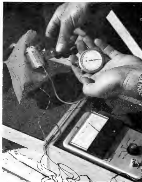
Resistance of a Thompson grape leaf to water loss, or diffusion, being measured by an autoporometer. The instrument, also called a diffusive resistance meter, indicates the amount of pores in the leaf's surface.
