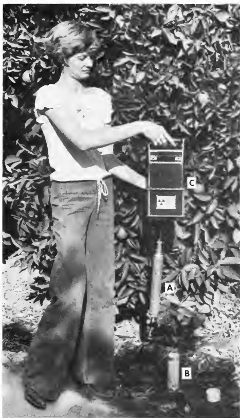
Neutron probe used to measure changes in soil moisture. The radioactive source of neutrons (A) fits into the access tube (B) leading into the ground. The probe (C) counts the neutrons. This instrument is used in agricultural research to determine how much water is being consumed by trees.
