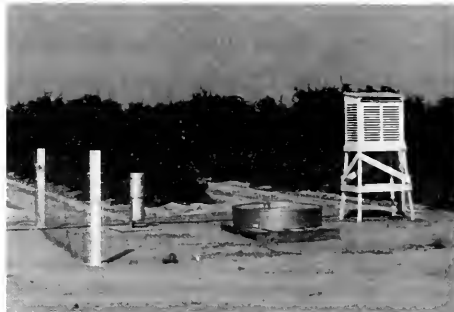
Agroclimatic station with evaporation pan containing water (center), rain gauge (left), and weather shelter, which holds instruments to measure air temperature and relative humidity. This station is recording climate data that relates the water consumed by the nearby orange trees to the rate at which water is evaporating from the pan.
