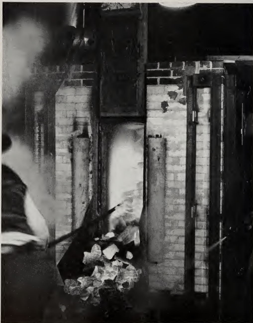
FIG. 1.—Discharging and quenching coke from slot-type experimental oven.
