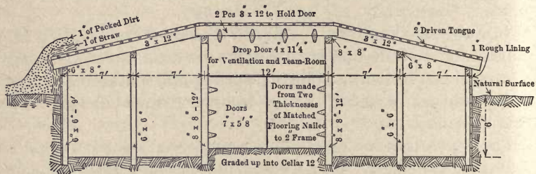
FIG. 66.—End elevation of a potato cellar.
