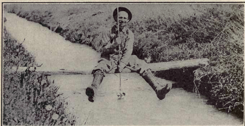
FIG. 54.—Measuring a canal with current meter.
