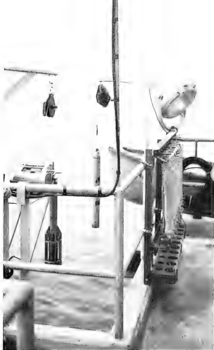
Bathythermograph lowered by an electric winch (left) provides detailed information on water column temperatures. Surface thermometer bucket (hanging from davit), Nansen bottles on rack, and floodlight are at right.
