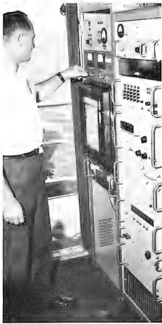
(Left) Recorders and other electronic equipments are mounted side-by-side in 19-inch racks along the south wall. (Center) The punch-tape recorders are used interchangeably and concurrently. They can be connected to a choice of several sensing instrument cables in the recording room. (Right) Fifty-two sensors transmit vertical and horizontal temperature readings to this analog recorder which is also connected to the adjacent punch-tape recorder.
