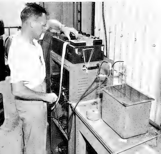
Measuring the sound attenuation caused by plankton with a resonant cavity chamber and recorder.
