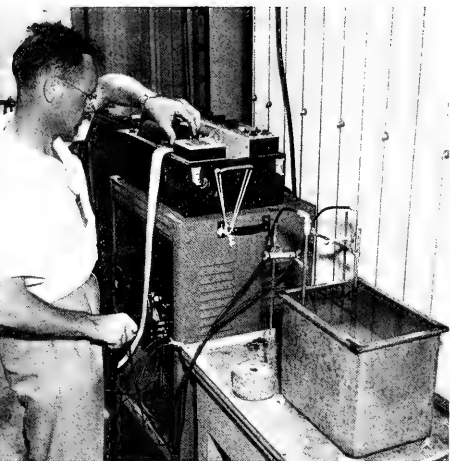
Scientist monitors resonant cavity equipment to measure sound attenuation caused by plankton organisms. Resonant cavity measurements require the tower's stable platform and proximity to fresh, live marine organisms.
