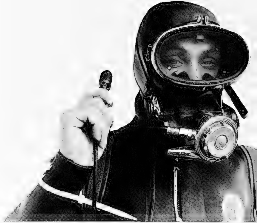
Communication equipment worn by the diver includes a special mouthpiece with microphone, a magnetic earphone, and a short length of cable attached to an underwater plug.
