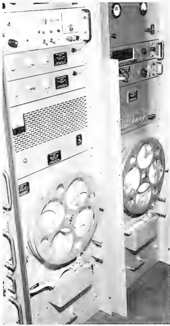
(Left) Recorders and other electronic equipments are mounted side-by-side in 19-inch racks along the south wall. (Center) The punch-tape recorders are used interchangeably and concurrently. They can be connected to a choice of several sensing instrument cables in the recording room. (Right) Fifty-two sensors transmit vertical and horizontal temperature readings to this analog recorder which is also connected to the adjacent punch-tape recorder.
