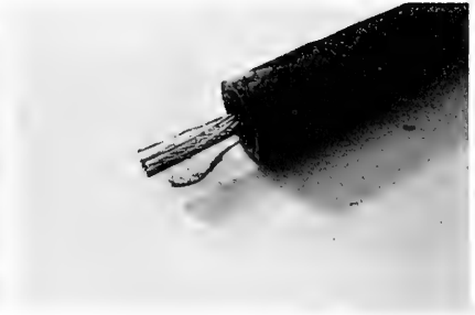
Figure 4-1. Failure of B-3540 Wire Rope Termination during Strength Test
