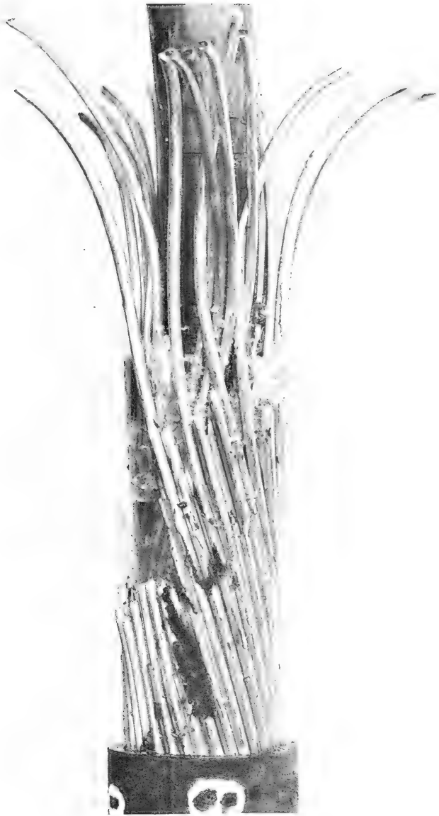
Figure 4-3. Armor Strands at Termination 4A. Parted at 15,000 lbs. Tension
