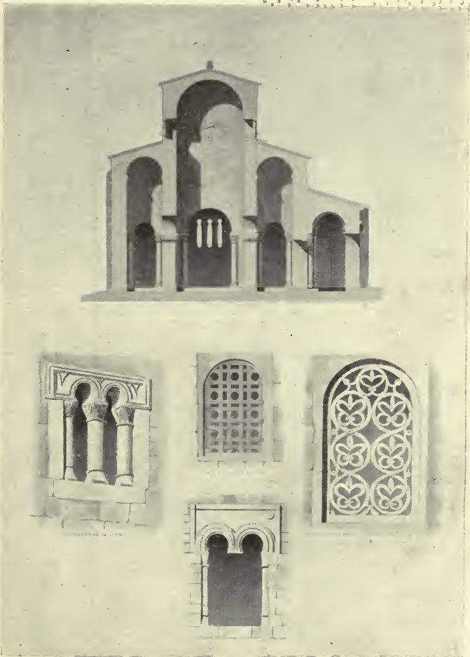
TRANSVERSE SECTION AND WINDOWS OF THE CHURCH OF SAN SALVADOR DE VALDEDIOS (CONCEJO DE VILLAVICIOSA) PROVINCE OF OVIEDO
