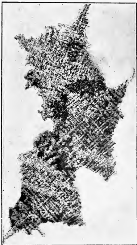
FIG. 21.—Sulphur print of a cross-section of three crystallites from a large steel ingot, showing the white skeleton crystals with sulphur trapped between the branches. Natural size. (Stead.)
