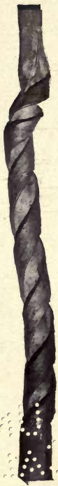
I-Beam Automobile Axle—Vanadium Steel— 3\frac{1}{2} twists in 24\frac{1}{2} inches. Elastic limit of torsion, 7,540 inch pounds.
