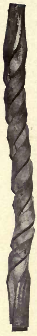
I-Beam Automobile Axle—Low Carbon, High Manganese Steel, treated— 3\frac{1}{2} twists in 24\frac{1}{2} inches. Elastic limit of torsion, 3,700 inch pounds.
