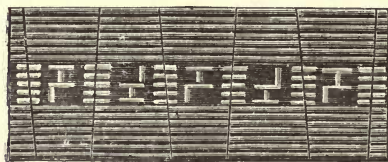
FIG. 71.—Divided plate by which 80 cakes can be made at a time in one press.
