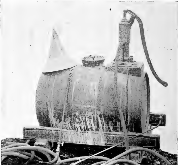
Figure 15.—Barrel spray pump, showing cone shaped strainer to the left.
