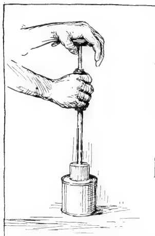
FIG. 358.—CAPPING A CAN WITH ROUND CAPPING STEEL
