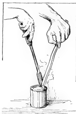
FIG. 359.—TIPPING A CAN WITH SOLDERING IRON AND SOLDER
