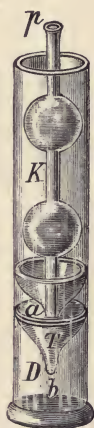
FIG. 2. Thorn's Extractor. D, Distillation Cylinder; K, Con- denser; T, Funnel; a, p, Condensing Tube.
