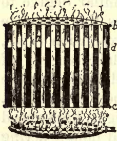
FIGURE 131. — Flue Boiler. This type of boiler consist of the crown sheets b c , connected by the tubes a a a , through which the fire is forced. The shell d is often wrapped with piano wire.
