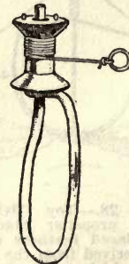
FIGURE 30.—Toy Helicopter. By rapidly pulling the string the propeller is revolved at such speed as to cause it to rise off the spool and ascend a considerable distance in the air.
