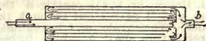
FIGURE 129.—Muffler. The gases entering at a flow back and forth as indicated by the arrows until they issue from the vent b .
