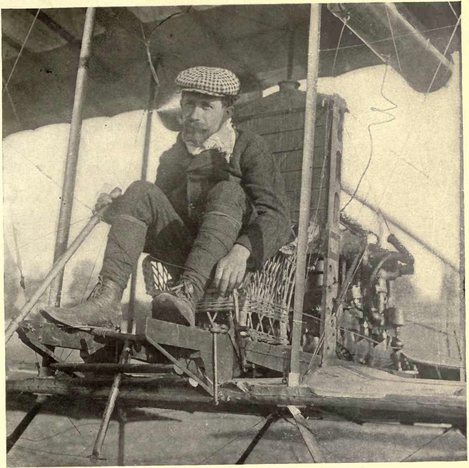
FIGURE 248.—Wicker Chair and Foot Control of Ailerons in Sommer's Farman Biplane.
