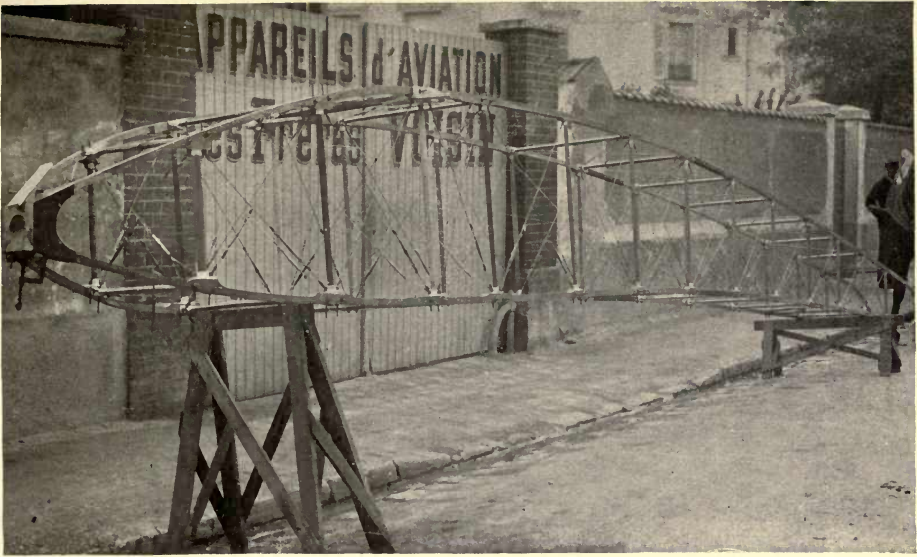
FIGURE 88.—Frame, or "Fuselage," of New Voisin Biplane. The ingenious use of wood, left of larger section at the points of attachment to the cross struts, which set into metal sockets, and the rigid diagonal wire bracing, constitute a peculiarly interesting example of modern high-grade aeroplane construction.
