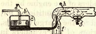
FIGURE 126. — Carbureter. Fuel from the tank flows through the pipe d until the float chamber c is filled to a level determined by the rising of the float a , which closes the valve b . From c extends a pipe terminating in the atomizing nozzle e , which is located in the pipe f , through which air is inspired in the direction of the arrows by the suction of the engine. This suction causes gasoline to spray from e in quantities proportionate to the force of the suction, except that at very high suction the valve g opens and by thus admitting air between c and the engine prevents the fuel from becoming too rich at high engine speeds. The butterfly valve at h is the throttle.
