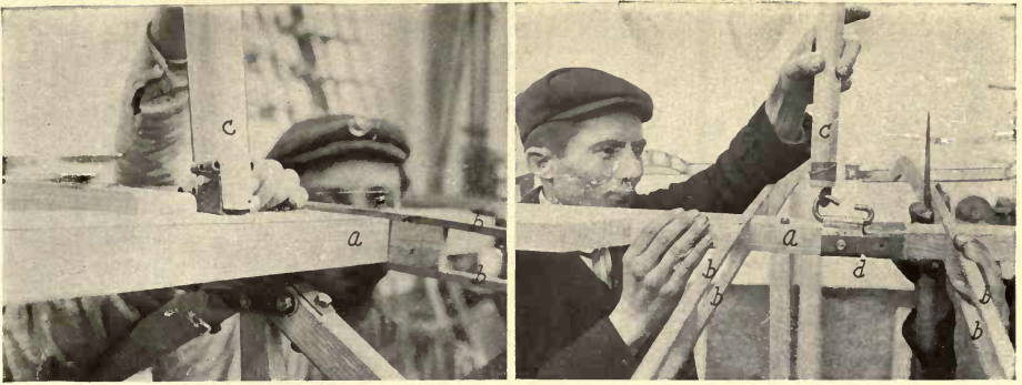
FIGURE 192.—Details of Wright Biplane Strut Connections. Note the manner in which the struts c are fastened in U-shaped metal sockets at the center of the machine and hooked to the wing bars a in the flexible wing ends. The plate d indicates the point at which the wings unship for convenience in shipping and storing, while b b are the double rib members.
