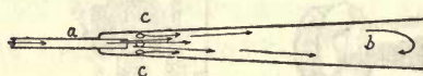
FIGURE 128.—Silencer. The gases entering at a induce an air flow in through the holes c c , with the result that by the time the exhaust reaches the mouth b it is contracted by cooling to a comparatively small volume.
