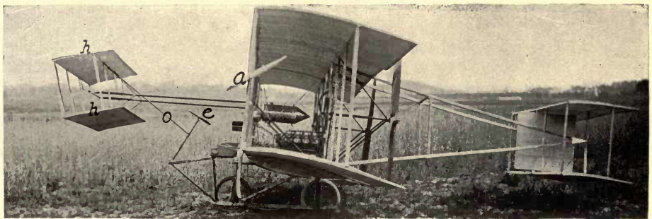
FIGURE 80.—Side View of Pischoff & Koecklin Biplane, showing one of the ailerons very clearly at a . The ingenious system of controlling the forward elevator hh by direct connection of the steering rod e to the steering pillar o is of interest.
