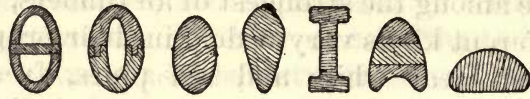
FIGURE 178.—Sections of Wooden Spars. The ends sought in these different constructions are light weight, great strength, and a minimum resistance to passage through the air.
