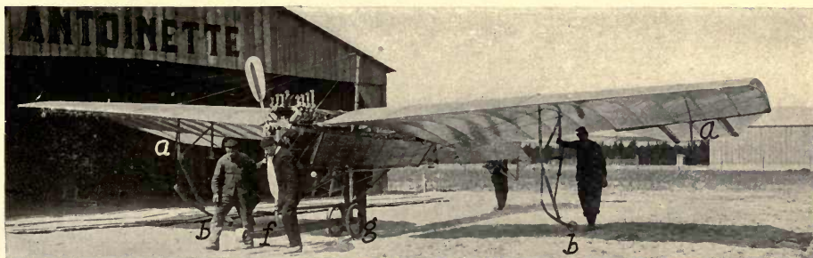
FIGURE 76.—Aileron Control of Lateral Balance in Antoinette Monoplane by manipulation of the two hinged tips aa .
