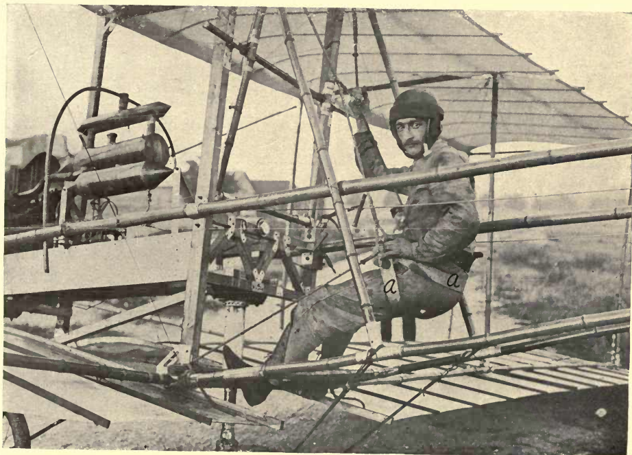
FIGURE 251.—Sling Seat of Captain Ferber's Biplane.
