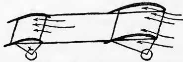
FIGURE 68.—Staggered Biplane. Note that the normal from the curves of the advancing edges meets the currents of upwardly-flowing air at right angles.
