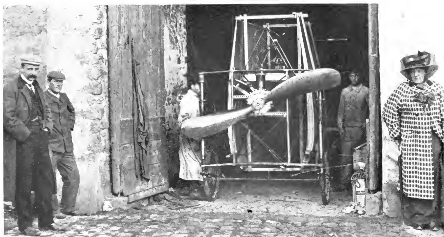
FIGURE 246.—Front View of Bleriot XI, Showing Demountable Wings.
