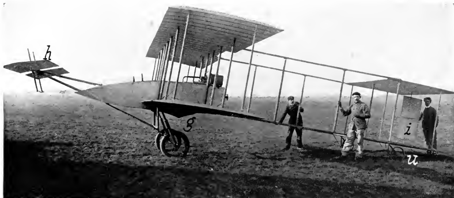
FIGURE 209.—Side View of Maurice Farman's Biplane. This machine resembles both the Voisin and the Farman machines—the former in its running gear and the latter in the absence of the vertical panels.
