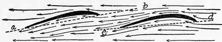
FIGURE 97.—Advancing and Following Surfaces. Showing the necessity for a different curve and steeper angle in the rear wing, that it may operate effectively through air disturbed by the front wing.
