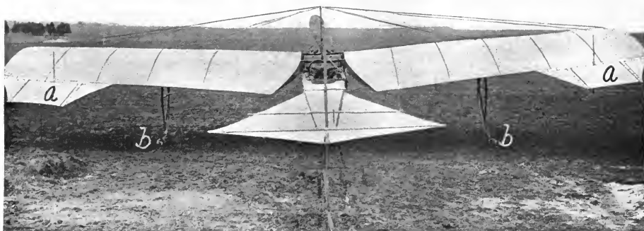
FIGURE 214.—Rear View of Antoinette V. In this view the ailerons a a and the balancing rollers b b are well shown.
