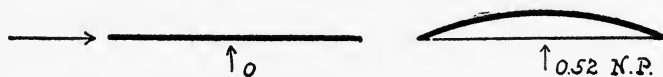
FIGURE 43.—Comparison of Plane and Arched Surfaces Without Angle of Incidence. Lilienthal found that while the lift of a flat surface placed as above was zero, the arc of a circle gave a lift equal to 52 percent of the pressure upon it when exposed in a vertical position to the same wind.
