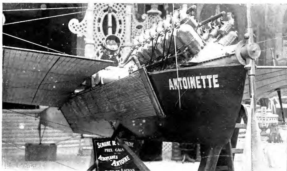
FIGURE 175.—Boat-like Body of Antoinette Monoplane. This machine, which is equipped with a hundred-horsepower motor, will run on the land, in the water, and in the air.
