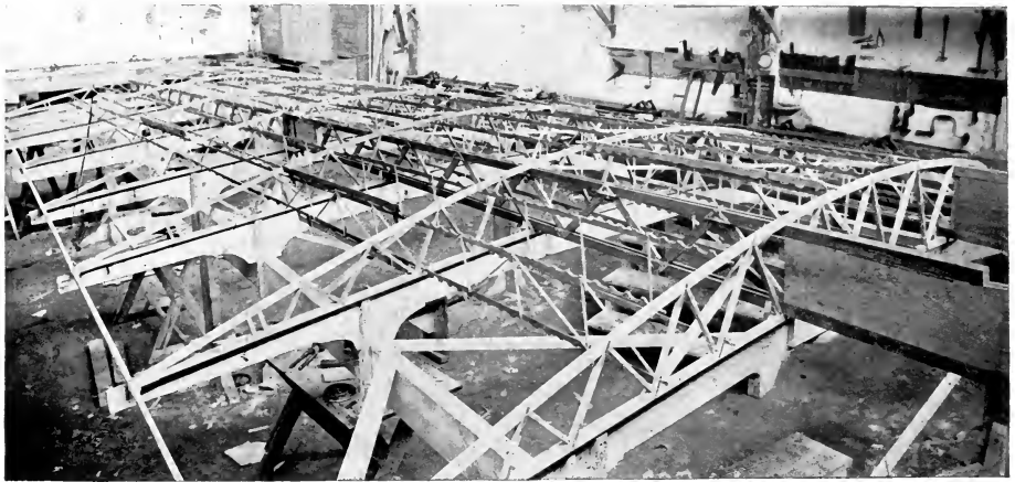
FIGURE 71.—Internal Framing of Antoinette Monoplane Wing.
