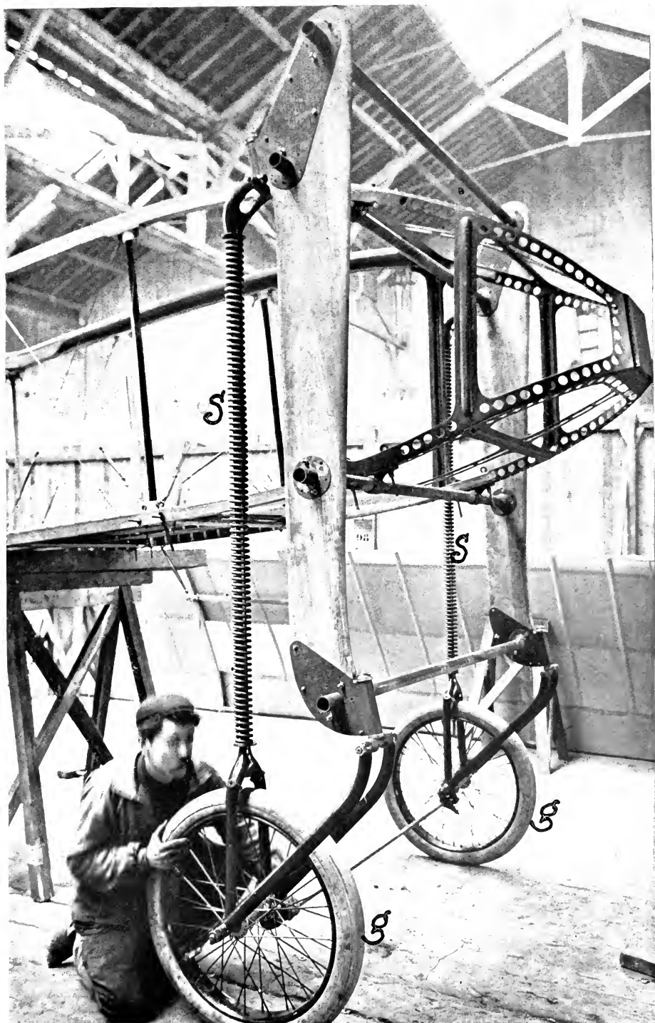
FIGURE 170.—Typical Alighting Gear. In this the upward swing of the wheels g g on their link connections is cushioned by the helical springs s s .
