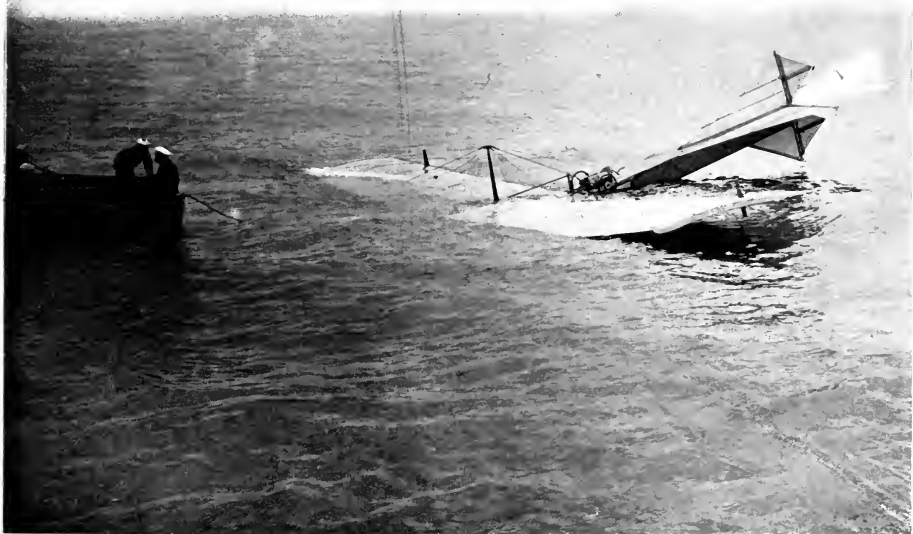
FIGURE 253.—Latham's Antoinette Monoplane in the English Channel. Showing that such a machine may be made to constitute an excellent raft.
