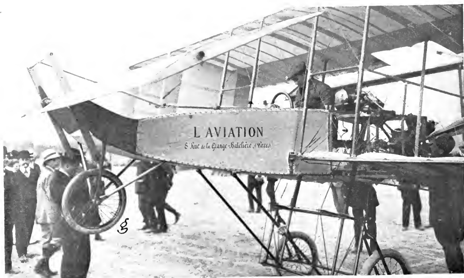
FIGURE 172.—Alighting Gear of Paulhan's Voisin. The wheel g on the proW is a safeguard against undue forward inclination of the machine in landing.
