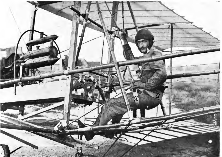
FIGURE 251.—Sling Seat of Captain Ferber's Biplane.
