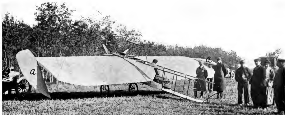
FIGURE 77.—Bleriot Monoplane VIII. The feature of this machine was the control of lateral balance by the pivoted allerons aa .
