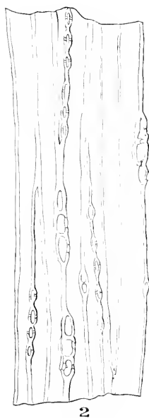
Fig. 46. Tangential section of wood of Pinus verba showing the medullary rays and pits in the walls of the wood-cells. \times 150 .
