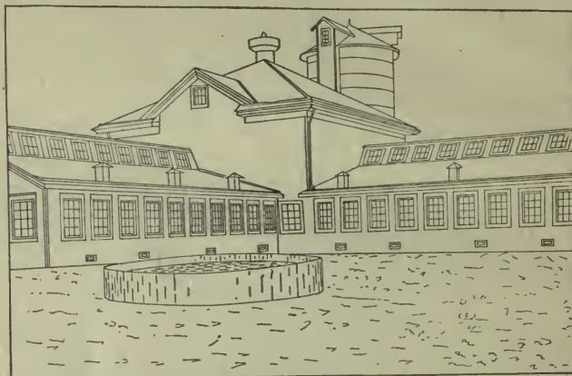
Fig. 34.—Showing faulty arrangement of windows for stables in cold climates, the effect being to render them cold and damp.
