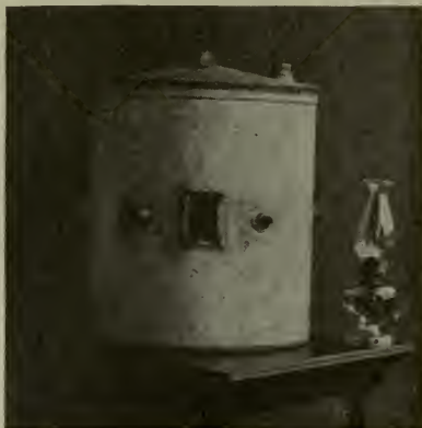
Fig. 14.—A ventilation chamber for observing the effects of inadequate change of air.
