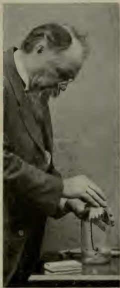
Fig. 13.—The candle in two quarts of air extinguishes itself in 30 seconds.
