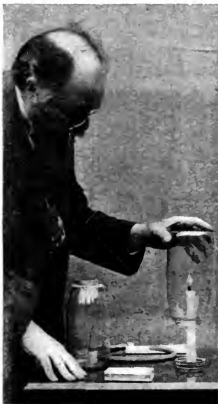
Fig. 30.—Respired air soon drops from the inverted jar and the flame is not extinguished.
