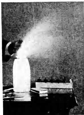
Fig. 7.—Magnesium ribbon burning in ordinary air.
