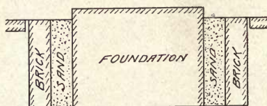
Fig. 66—Foundation to Prevent Vibration
