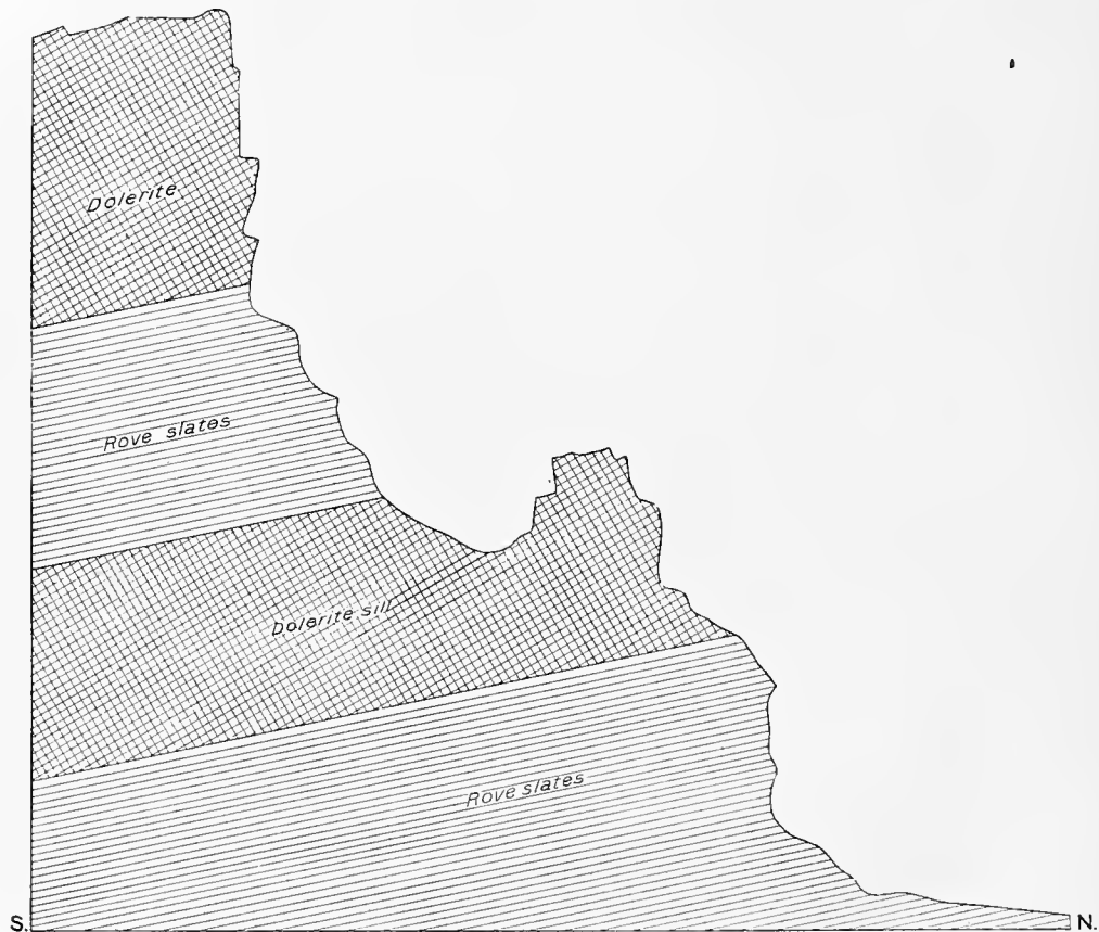
FIG. 22.—Section through the Rove slates, with intercalated Logan sills south of Gunfint Lake.
