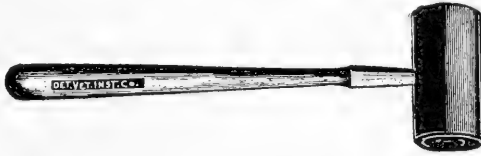
34.—Rawhide mallet. This instrument is smaller and lighter than a wood mallet and is used for the same general purpose.
