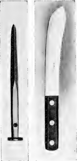
Fig. 5.—A, butcher knife with cutting edge in direct line with the handle, leaving no heel to catch in the tissue when making long incisions. Very useful when proper instrument is not available. B, with. Very useful for destroying large animals.
