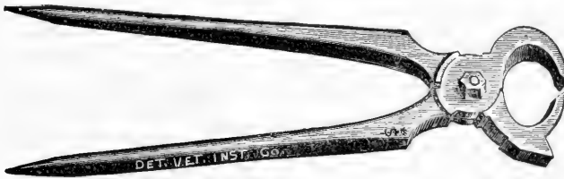
FIG. 35.—Iron pinchers for removing sole and wall of hoof.
