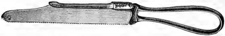
FIG. 52.—Charriere's blade saw. This instrument is used in work on the nasal and cranial bones of small animals.
