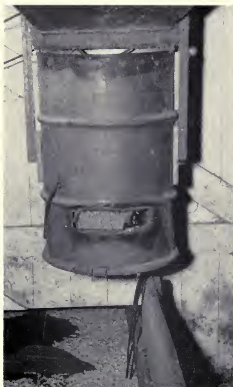
The top half of this barrel is a hopper for ground feed. A vibrator-type feed meter in the bottom half delivers the feed at the correct rate to the push-pull type bunk feeder. (Fig. 2)
