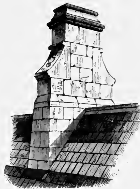
DESIGN FOR CHIMNEY WITH VENTILATING FLUES.
