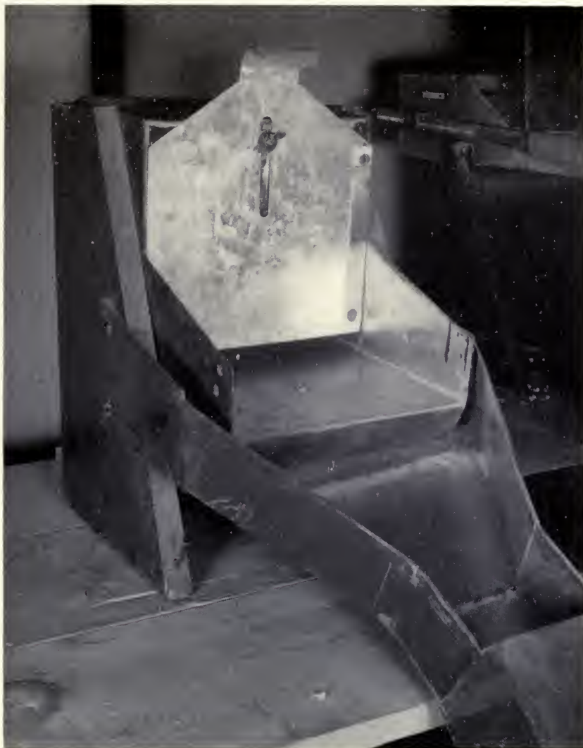
This vibrator meter consisted of a metal box with a 120-volt, 60-cycle AC vibrator attached to the bottom. Previous tests 10 indicated that this particular type of vibrator unit would satisfactorily operate at line voltage and that the capacity could be regulated by adjustment of a gate in the discharge trough. For these tests, line voltage was used on the vibrator and all capacity adjustments were made with the gate. (Fig. 6)
