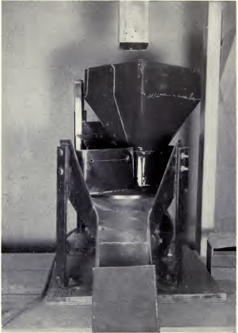
This rotating table meter consisted of a 12-inch flat disk powered by a 36 r.p.m. gear motor. The capacity was regulated by adjusting the height of the grainspout above the disk top. The spout was centered on the disk. (Fig. 3)
