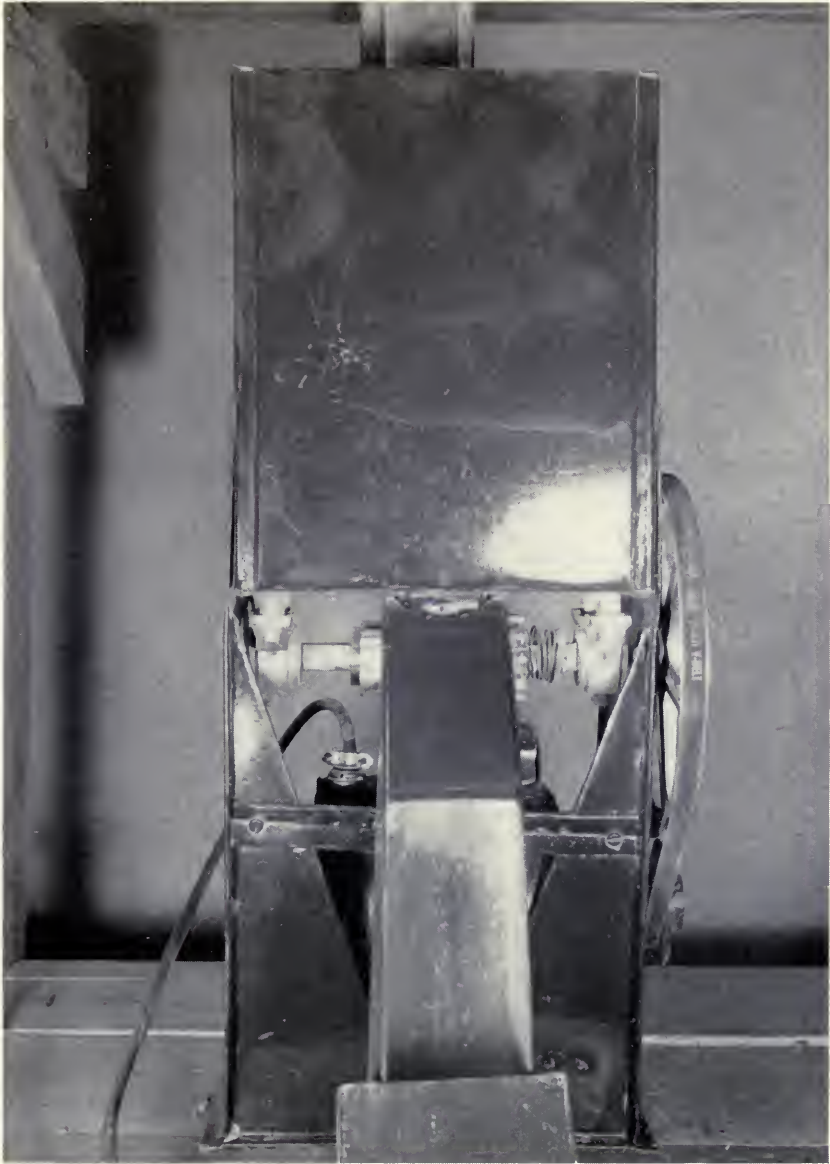
This fluted wheel meter consisted of a small fluted wheel unit taken from a small-grain drill. It was driven at 450 r.p.m. to achieve the desired volume. Its capacity was regulated by sliding the fluted wheel in and out of the well at the bottom of the feed hopper. (Fig. 2)
