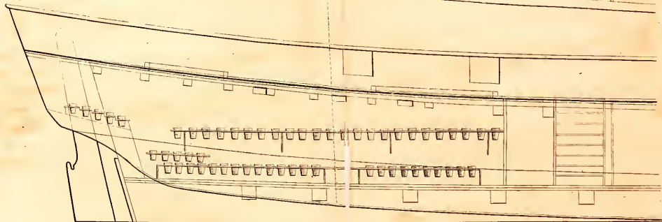
PLAN & SECTION of part of the BOUNTY ARMED TRANSPORT, showing the manner of fitting and stowing the lotts, for receiving the Bread-fruit plants.
