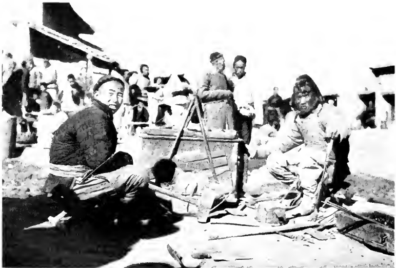
An itinerant blacksmith-shop, with the box-bellows worked by a stick handle widely used by craftsmen and cooks in China
