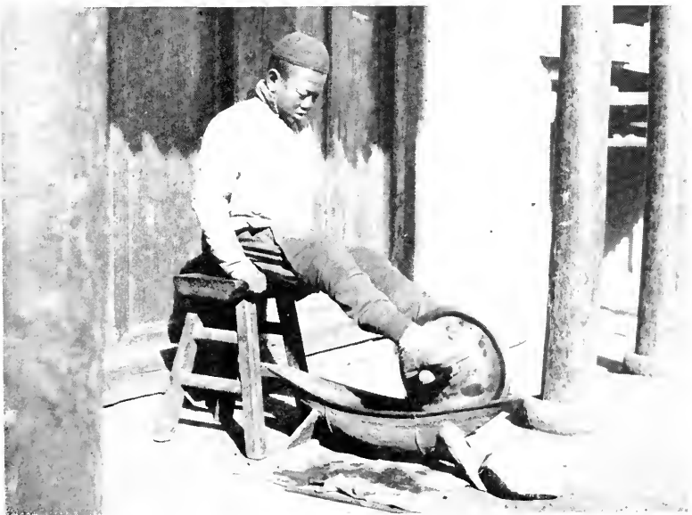
This method of grinding up red peppers and the like is wide-spread in China. Both trough and wheel are of solid iron
