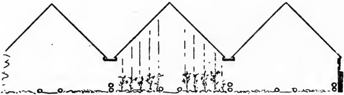
FIG. 54.—Arrangement of span houses and piping for tomato growing for the market.
