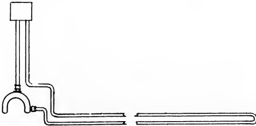
FIG. 16.—A means of obtaining a circulation through pipes wholly below boiler level.
