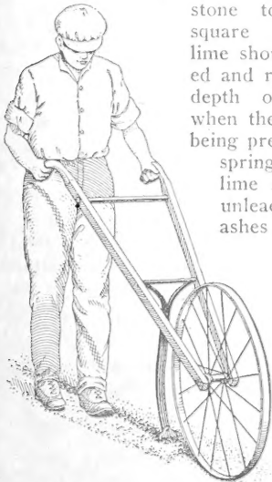
Fig. 3—Wheel hoe or hand cultivator. This can be had with various attachments, such as plow, cultivator teeth, shovels and rake. A simple form may be made at home.
