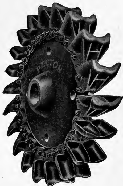
Fig. 166.—Pelton Tangential Water Wheel Runner. Designed for 5000 H. P. at 865 foot head and 225 R. P. M. (Pelton Water Wheel Co.)
