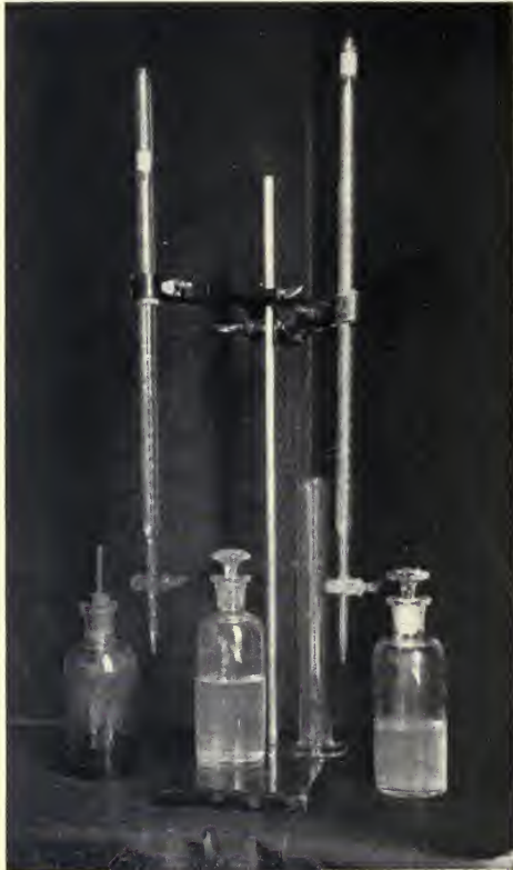
FIG. 62.—Apparatus for Alkalinity Test.
