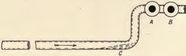
Fig 27.—Dangerous pipe arrangement.
