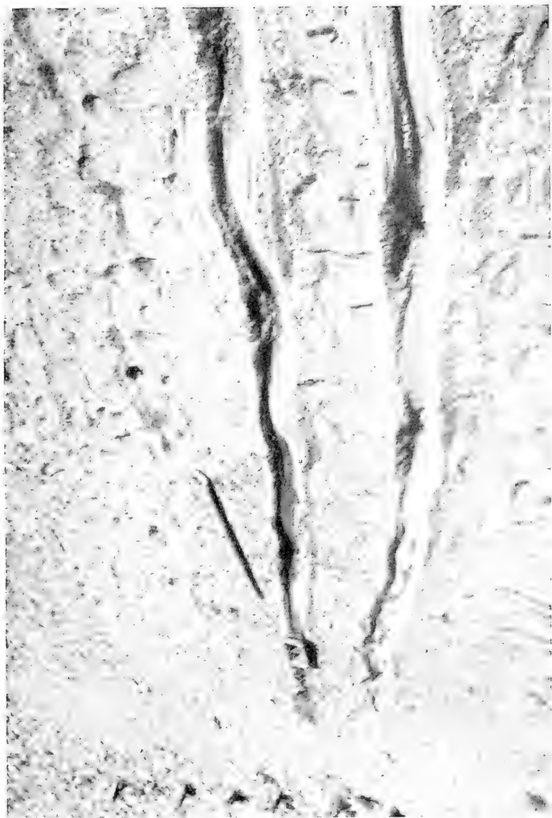
PLATE 50.—Undulations made by a model sledge drawn slowly and steadily through slightly moist sand.
