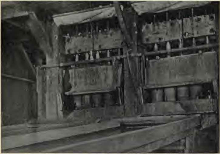
FIG. 103.—THE STAMPS IN A QUARTZ-MILL
