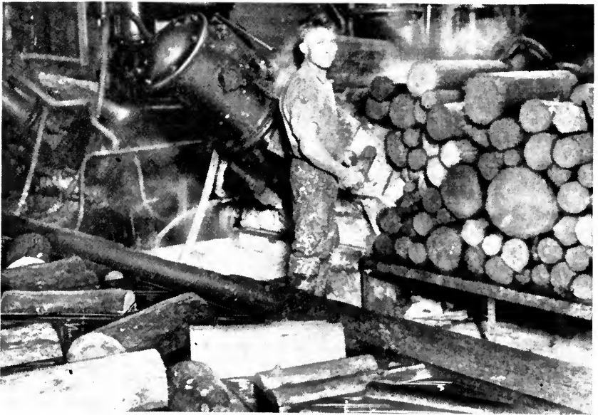
WORKMAN putting logs into a box-like opening in a turret of a grinding machine. When he closes the door a pneumatic piston will force the logs under tremendous pressure against the stone. Hot, white slush of ground wood is seen flowing out just behind the workman.
