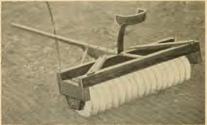
Fig. 18.—A successful cement, home-made roller.
