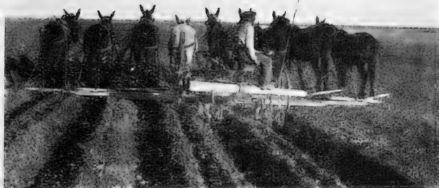
Fig. 8.—A two-row lister with eight horses listing from eight to nine inches deep, Hays, Kas., Experiment Station.
