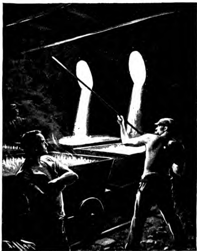
DRAWING THE BLACK ASH FROM A REVOLVING FURNACE.
