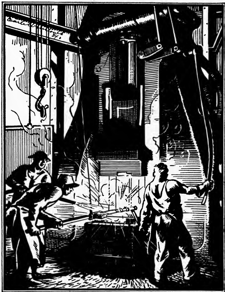
The trip-hammer drops on to the crankshaft.
