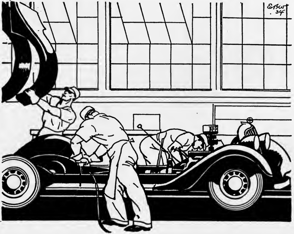
The men bolt on the fenders and running boards.
