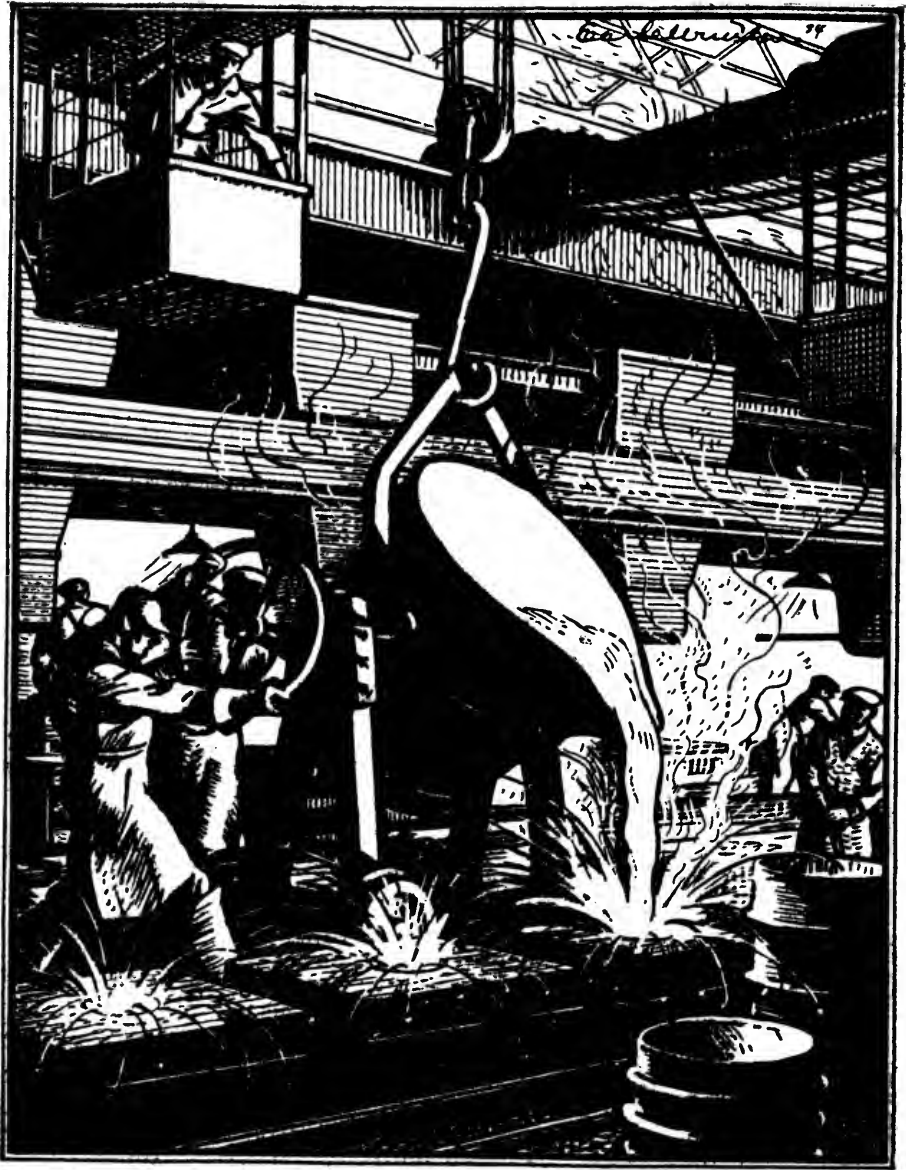
The men pour the hot metal into the molds.
