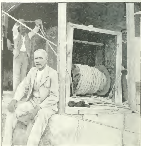
"BEHIND THE SCENES" UP IN THE CATHEDRAL TOWER—HERE WE SEE THE MECHANISM BY WHICH THE ANGELS, ETC., ASCEND AND DESCEND TO FROM THE STAGE BELOW. [Photo.]
