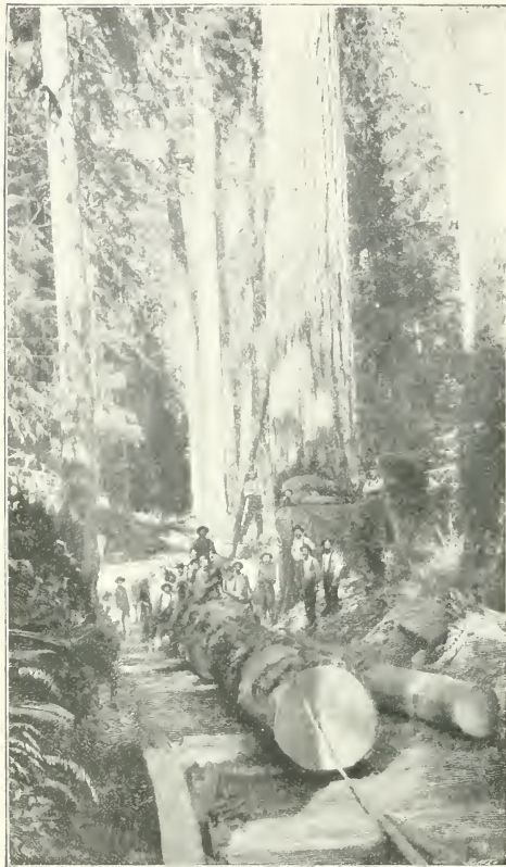
LOGS BEING HEALED DOWN A "SKID" ROAD — FELLEES AT WORK IN THE BACKGROUND.
