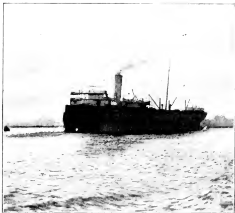
11.—THIS SHIP WAS WRECKED, BUT THE ENTERPRISE SALVAGERS CUT OFF THE REAR HALF, TOWED IT TO PORT, AND BUILT A NEW FOREPART ON TO IT. From a Photo.
