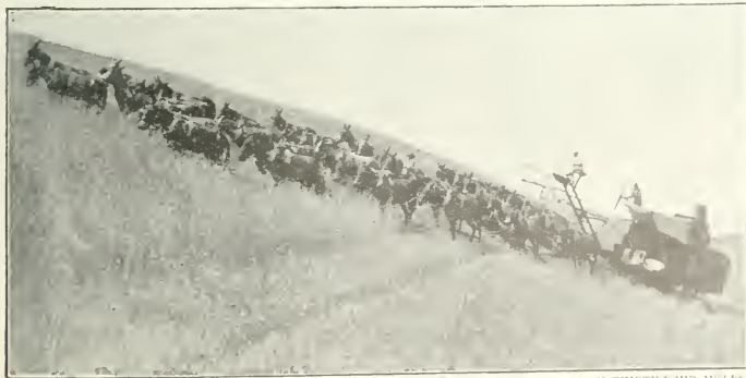
A GIGANTIC REAPING-MACHINE AT WORK IN THE SACRAMENTO VALLEY—IT IS DRAWN BY THIRTY-FOUR MULES AND ONLY REQUIRES THREE MEN TO LOOK AFTER IT. [Photo.]
