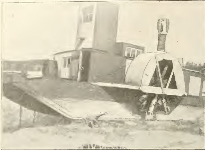
A CANADIAN "ALLIGATOR BOAT." IT CAN TRAVEL BOTH ON LAND AND IN THE WATER. From a Photo.
