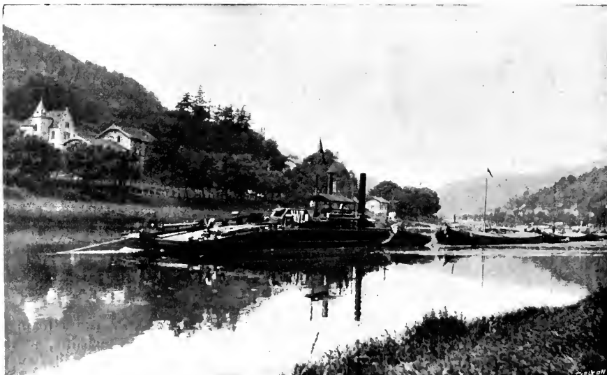
ONE OF THE EXTRAORDINARY NECKAR STEAMBOATS—THEY PULL THEMSELVES ALONG BY HAULING UP A CHAIN LAID ALONG THE BOTTOM OF THE RIVER.
