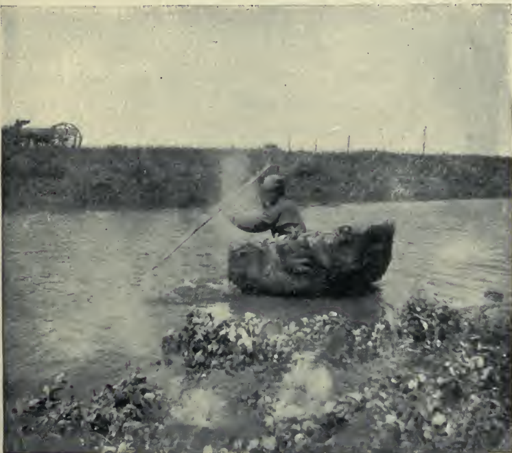
Boat Made of Framework of Sticks Covered with Bison- or Horse-hide. Frequently Used in Early Days of the West.
