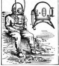
Diving-dress and Diving-helmet by Stebe, Gor-man & Co.---a, Pipe by which air is supplied; ô, valve by which it escapes.
