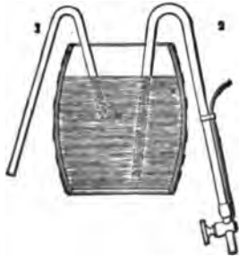
1. Common Siphon. 2. Improved Siphon, with exhausting tube for filling it.
