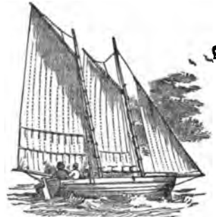
Wherry with fore-sail reefed, the main-sail showing reef-bands and reef-points.
